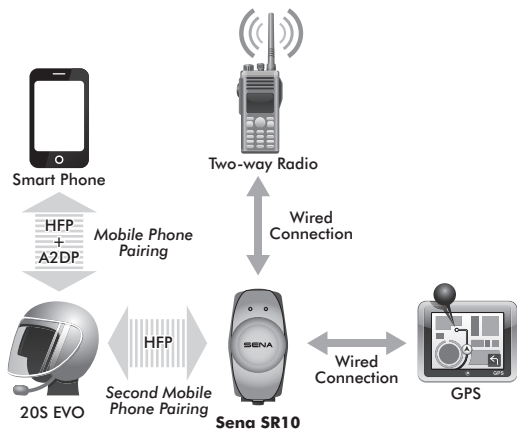
Parallel Connection of SR10 and Mobile Phone by Bluetooth Second Mobile Phone Pairing
