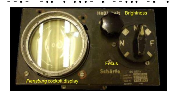
*Flensburg* was a threat receiver fitted to Luftwaffe night-fighters in Spring 1944, and tuned to the 300 MHz emissions of the RAF *Monica* tail-warning radar. It had good sensitivity and angular discrimination, and enabled the fighter pilot to pick out a single bomber even in a stream, radiating multiple *Monica* signals.
