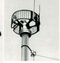
Newer U-boat mounted *Bali* circular dipole (90-470 MHz).
