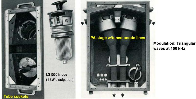
Arrows: cooling air for grid circuit & output coupling loop
