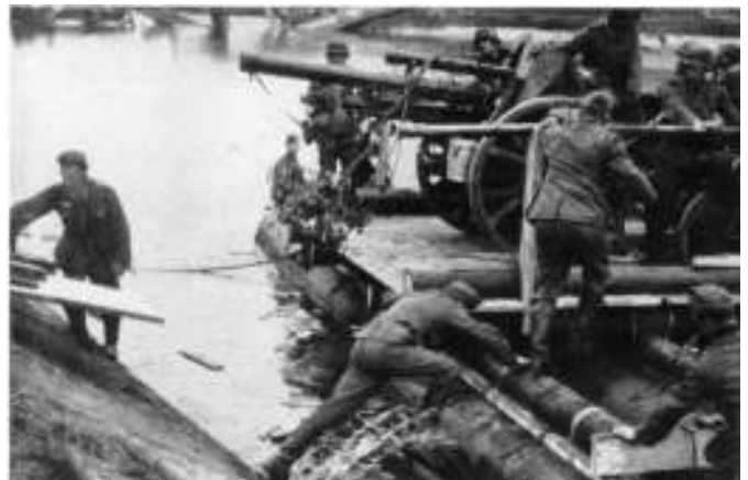
A large rubber-boat ferry with a IFH 18 loaded on it sets out from the shore; in the background is a blown-up bridge.
