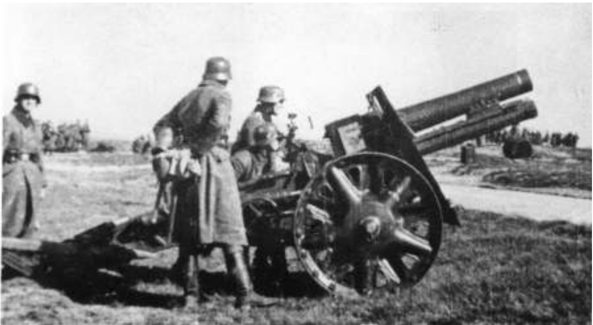
A heavy infantry gun in firing position, being aimed with a panoramic scope.
