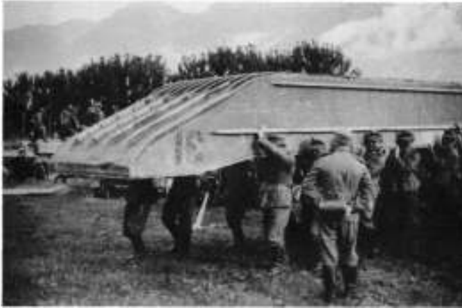
A half-pontoon is taken to the water after being unloaded (a drill photo from Germany).
