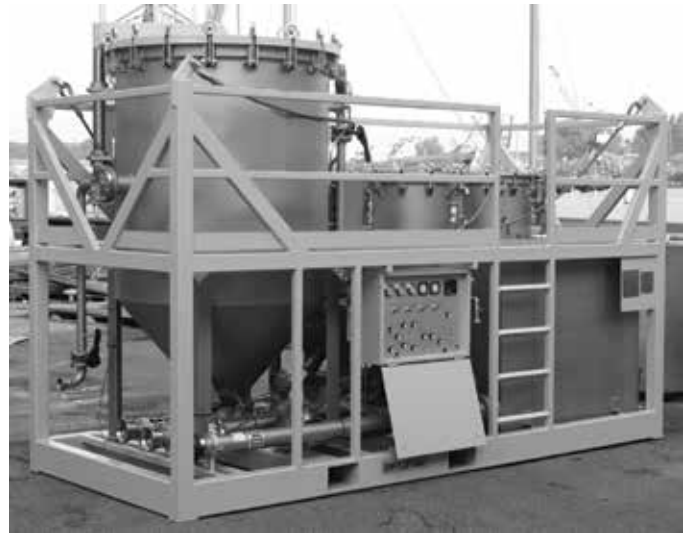
The self-contained Weatherford combination VPL/cartridge filter unit has many safety features, including railings, a ladder, and a service platform.
