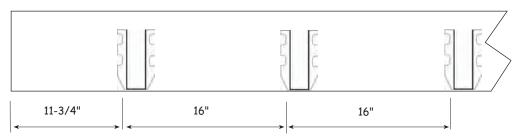
2. Measure and mark the hanger locations on the opposite wall. **IMPORTANT**: Place the hangers to the left of these marks. Floor joists should be parallel to the 16' wall.
