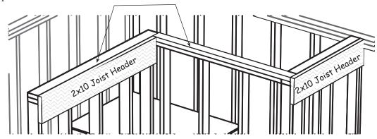
2. Cut, from a 12' long 2x10, to length and install as joist headers on the 68-1/4" and the 39-1/2" long wall frames, flush with the top of the tie plate. Use 10d sinkers as described previously.
