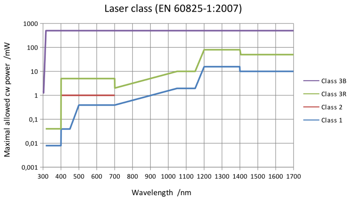
Figure 3.1: Maximal allowed continuous wave power as a function of wavelength. Chart by Danh, CC BY-SA 3.0, en.wikipedia.org/wiki/Laser_safety
