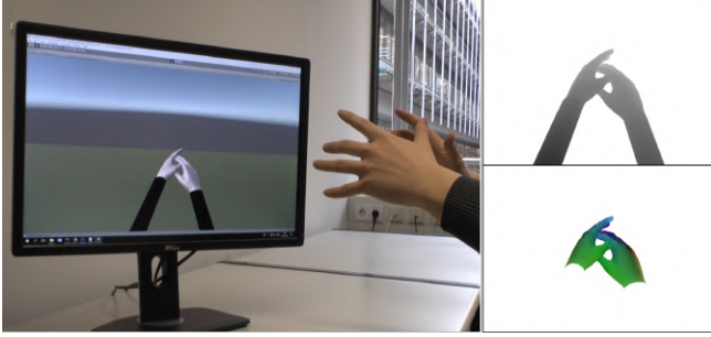
Fig. 4. We generate our synthetic dataset by tracking two hands, separated by a safety distance, which are used to control in real-time a physically-based simulation of two interacting hands in the virtual scenario (left). We output the depth map (top right) and dense surface annotations (bottom right) of the resulting simulation.
