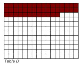
By default, the location of the last cluster at the time that you create an image determines the minimum amount of free space that must be available on the hard drive to which you intend to restore. In this example, assuming the partition size was 100GB, you would not be able to restore it to a space smaller than 75GB.
