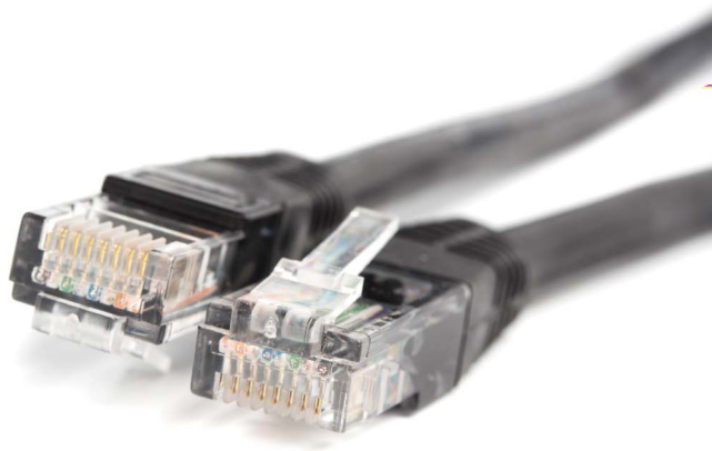
LAB FIGURE 13.5 Verify the color codes on both connectors
