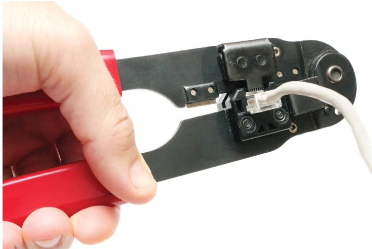
LAB FIGURE 13.3 Crimp the RJ45 connector firmly
