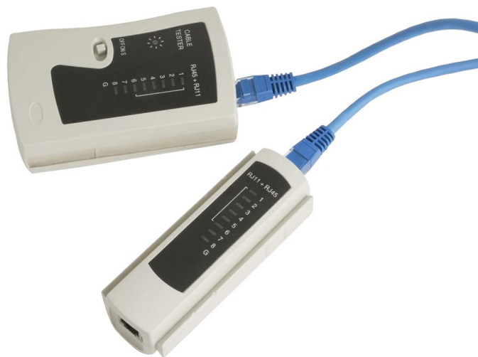
LAB FIGURE 13.4 Network cable tester
