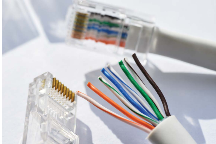
LAB FIGURE 13.1 Strip the cable sheathing
