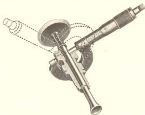
Fig. 29—Checking Valve Guide Bushing for Wear
