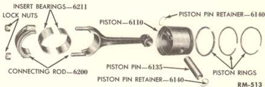
Fig. 17—Connecting Rod and Piston Assembly, Disassembled
