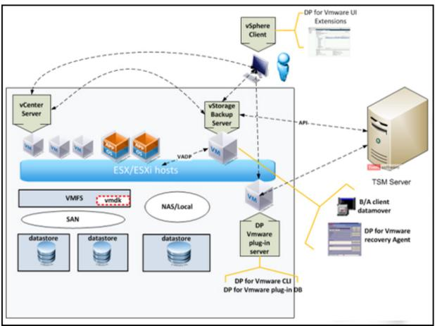
Figure 2. Data Protection for VMware components overview
