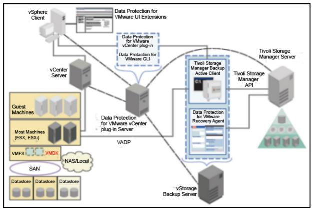
Figure 1. Data Protection for VMware system components and user environment
