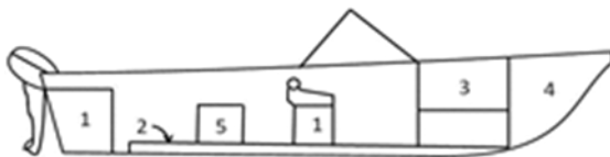
Figure 1 showing compartments where vapors may become trapped.
