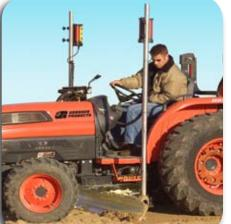
Grouser Products offers two laser control options for the Belly Blade. Laser controls along with the Belly Blade provide greater efficiency in both fill materials and time to complete a project.
