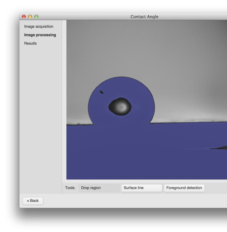
The image processing window requires you to define the 'drop region' and 'surface line' of the image. Click on the 'Drop region' button in the 'Tools' panel then drag over the image preview to define the region. Similarly, click on the 'Surface line' button and drag a line to define the surface that the drop is sitting on. With the 'Surface line' button depressed and the preview widget focused, use the arrow keys for finer adjustments of the surface line.
