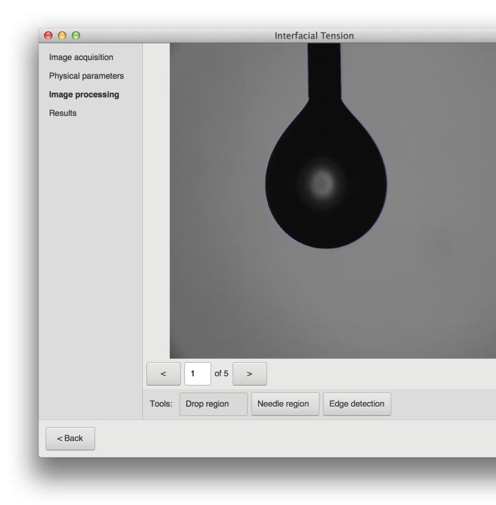
The image processing window requires you to define the 'drop region' and 'needle region' of the image. Click on the 'Drop region' or 'Needle region' buttons in the 'Tools' panel, then drag over the image preview to define the associated
