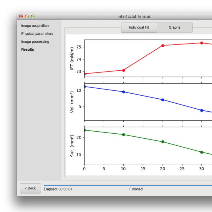
The 'Graphs' view shows plots of interfacial tension, volume, and surface area over time.
