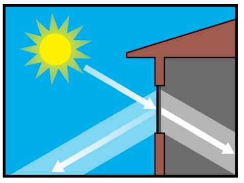
**Solar Heat Gain Coefficient**
