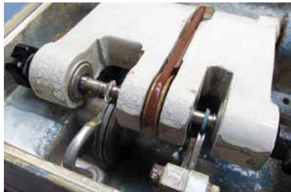
Custom cut crystal ground to match bezel mold.
