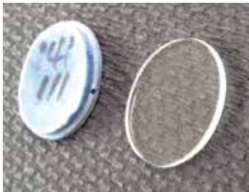
Mold of Bezel and crystal cut from it.
