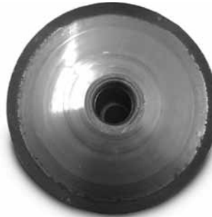
sliding flange before cleaning
