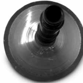
fixed flange before cleaning
