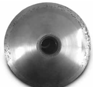
sliding flange after cleaning
