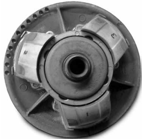
Pulley with the cap are removed
