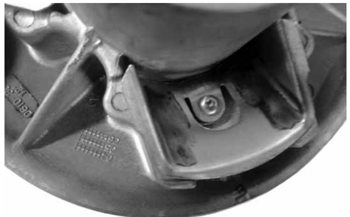
the sliding flange ramps once cleaned
