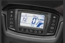
The smart new meter panel alerts you to all major vehicle functions with seatbelt and parking brake alarms and overheating and intermediate gear control indicators. The modern white LCD display provides excellent visibility at all times, even under difficult lighting conditions.
