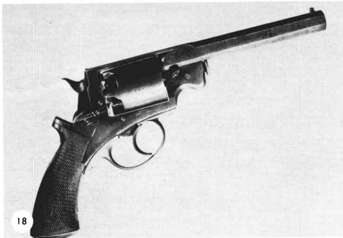
18. Adams patent Navy size revolver, serial no. 405, with lanyard ring on the butt and the different backstrap and checkering pattern.
