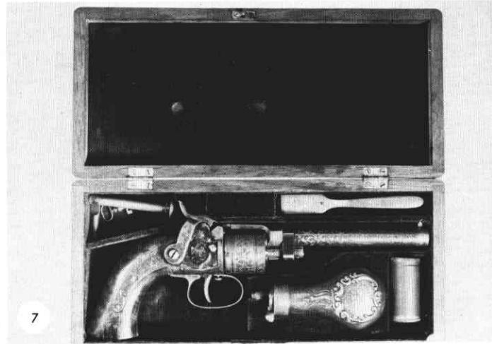
7. Belt size hand revolved revolver in original case again showing the proper accessories. The acid etched barrel is very unusual. The cylinders on all of these revolvers were acid etched, but to find it on any other part is unusual.
