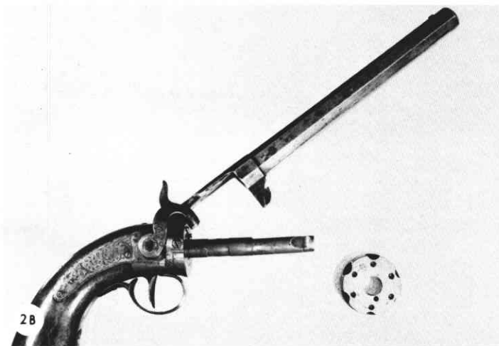
2a A pre-production type belt revolver and a (2B) dragoon revolver of production type with the barrels raised to show the difference in catches.
