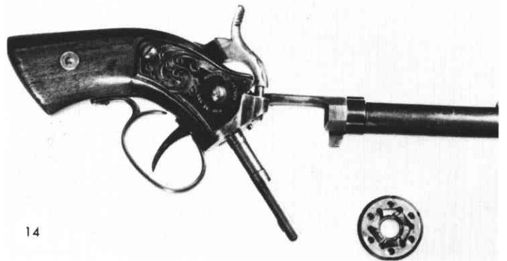
14 Rear of the cylinder of the Stevens 1855 patent revolvers. The holes around the periphery of the cylinder are the flash holes for discharging the chamber, the large holes are the cylinder stops, while the inner ring is the ratchet for turning the cylinder, this ratchet is the same whether it is revolved by cocking the hammer or pulling the trigger.
