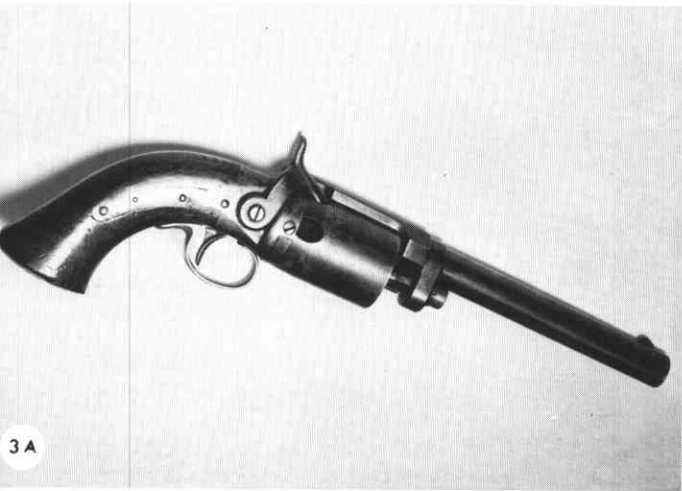
3A The dragoon size Wesson & Leavitt revolver, six-shot, .40 caliber, and approximately 4 lbs. About 1,000 were made.
