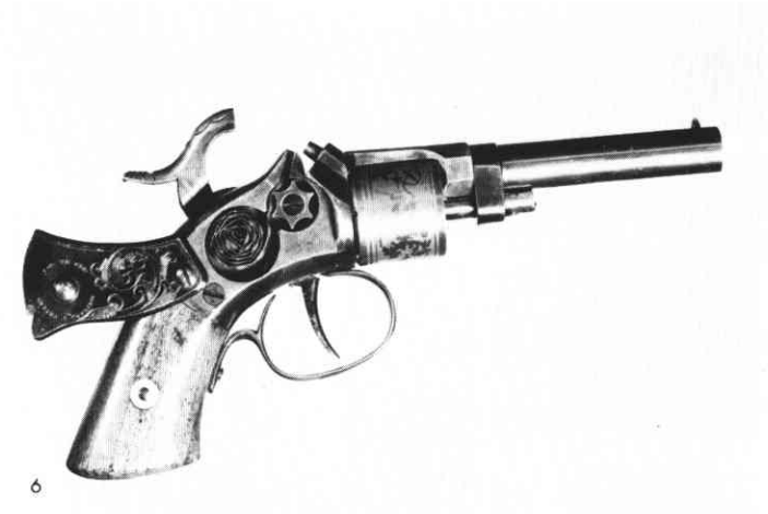
6 The Maynard tape priming system showing the roll of caps. Just like today's cap guns, they are advanced by the roller, which is operated just like the cylinder on a normal revolver. The cap is cut off individually as it is fed through the notch in the top of the lock plate and smashed against the nipple.
