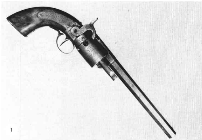
1 A belt size Wesson & Leavitt revolver of the preproduction type with an octagonal barrel and no markings, probably made in Europe.
