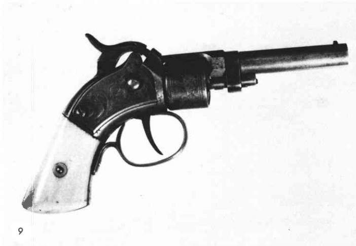
9. Stevens 1855 patent revolver with convex cylinder face and revolved by pulling the trigger. After pulling the trigger the first time to revolve the cylinder the hammer is then cocked and a second pull on the trigger fires the gun.
