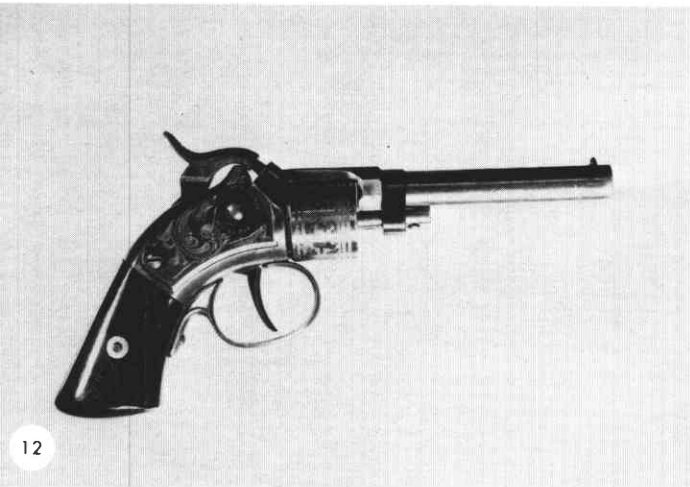
12 Stevens 1855 patent pocket revolver, flat cylinder face, hammer revolved, 3 inch barrel.
