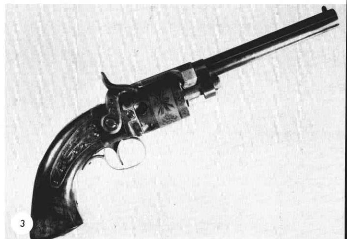
3 Belt size Wesson & Leavitt revolver, showing the use of the Stevens patent barrel catch, which rotates around the main barrel and hooks over the cylinder pin to hold the barrel in place.
