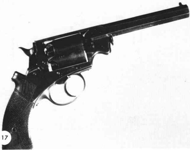
17. Standard production Adams patent Navy size revolver with lanyard hole through the grips, serial no. 987, nearly at the end of production.
