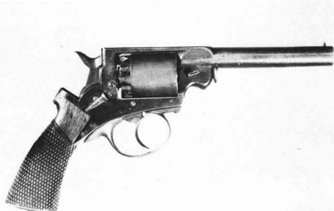
20. The Adams patent pocket size revolver with a 4 inch round barrel. Only about 200 of these round barreled pocket revolvers were made.
