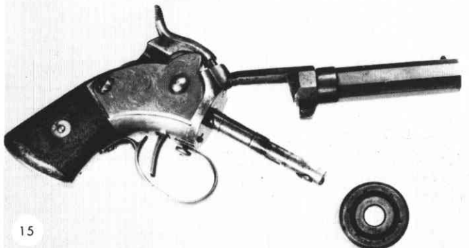
15 Rear of the cylinder for the hand revolved revolver showing the differences between it and the self cocking type. These have no ratchet for turning, only the notches the spring loaded catch goes in.
