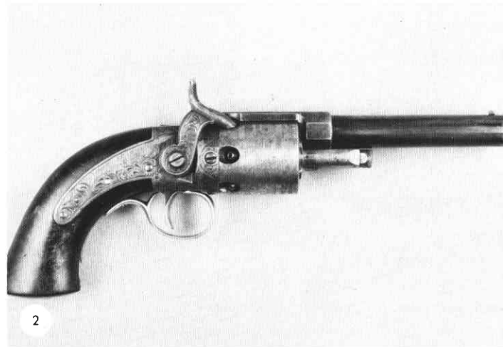
2 A belt size preproduction revolver made by the Massachusetts Arms Company. The barrel is released for removing the cylinder by pulling forward on the knob at the front end of the cylinder pin. Sam Smith collection.
