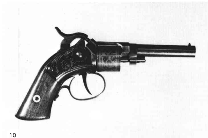
10. Stevens 1855 patent pocket revolver, serial no. 15 revolved by the hammer, flat cylinder face and 3 inch barrel. This was converted from the trigger revolved type by making some internal changes, the only external change is the addition of a set screw at the rear of the trigger, this kept the trigger from being pulled too far.
