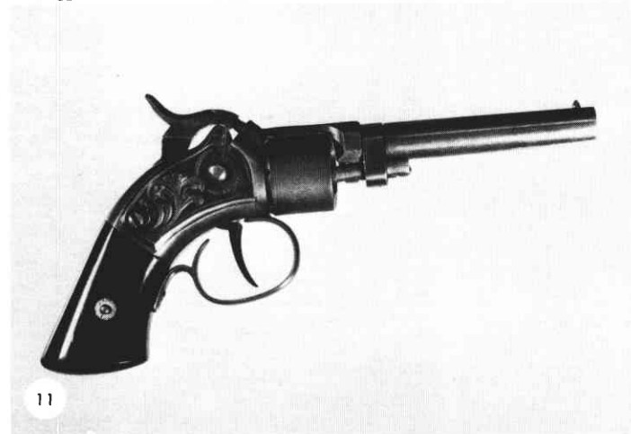
11. Stevens 1855 patent pocket revolver, serial no. 398, with a convex cylinder face and revolved by cocking the hammer, 3½ inch barrel. Note also that this gun has serial no. 1005 on the bottom of the barrel. These pocket revolvers may have as many as four different serial numbers on them, which are not serial numbers at all, but a means of keeping track of the patent royalties due the various patentees.
