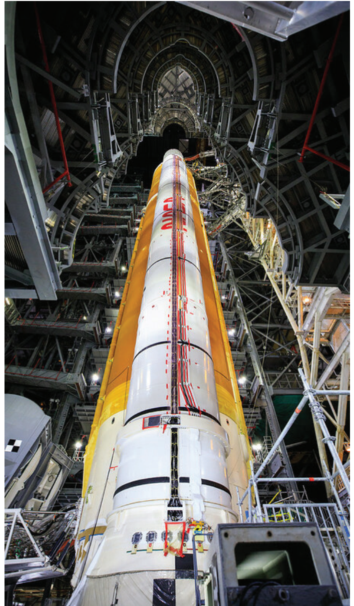
Artemis I boosters and core stage in the Vehicle Assembly Building at Kennedy Space Center in Florida (side view).
