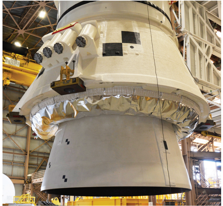
The aft assemblies of the Artemis I boosters on the mobile launcher in the Vertical Assembly Building.
