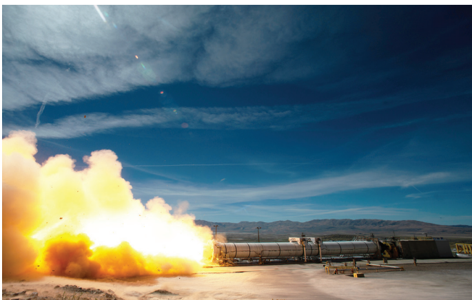
Flight Support Booster-1 (FSB-1) underwent a hot fire in September 2020 to evaluate materials and processes for future missions.
