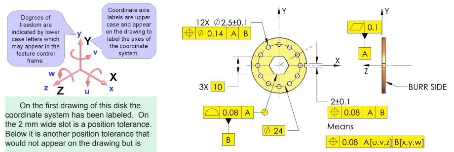
The function of the hex is only to transmit torque. Design does not want the hex feature to control the orientation of the datum reference frame. The 12 holes need to be oriented relative to the width of the 2 mm slot. Design would like to orient the datum reference frame using the width of the 2 mm slot. There was no way to do this in past Y14.5 standards. By customizing the datum reference frame, the design intent may be achieved.
