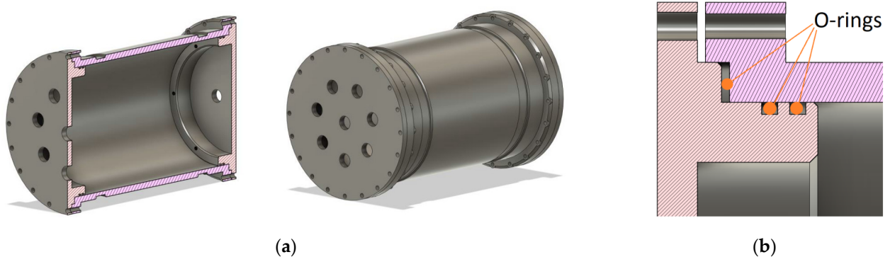
Figure 6. (a) Hermetically sealed unit for electronics; (b) O-rings of the hermetically sealed unit.
