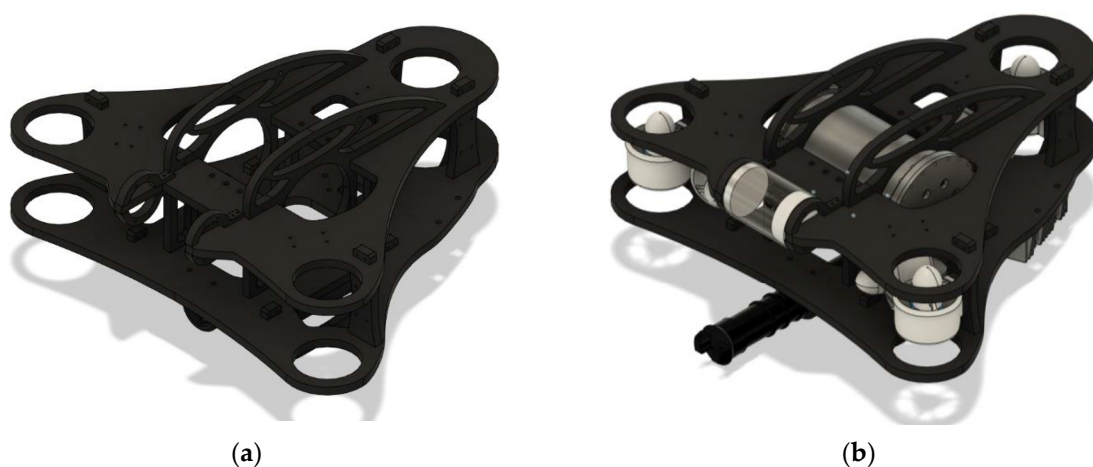
Figure 5. (a) Three-dimensional (3D) model of SevROV frame; (b) 3D model of assembled SevROV.
