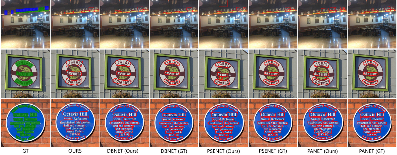
Figure 4. Visualization results of training using the generated polygons. The green-filled polygons are the ground truths, the blue-filled polygons are the ground truths that are marked as “don’t care”, and the red polygons are the detection results. Method (GT) represents training using the polygons generated from GT points; while Method (Ours) represents using the polygons generated from existing single-point text spotter (SPTS v2). Best view in screen.
