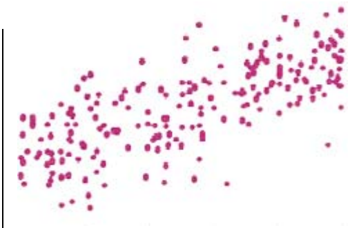
Broader spread of x -values ( s_x \uparrow ) Smaller Standard Error, SE(b_1) \downarrow
