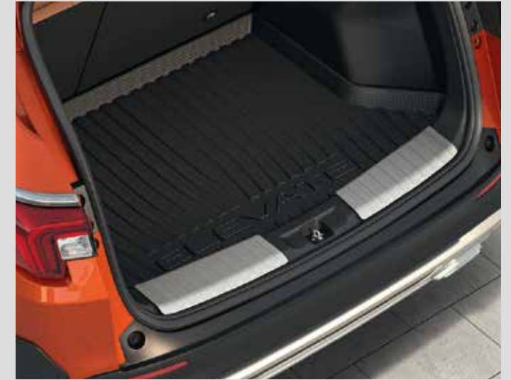
Tail Gate Entry Guard
