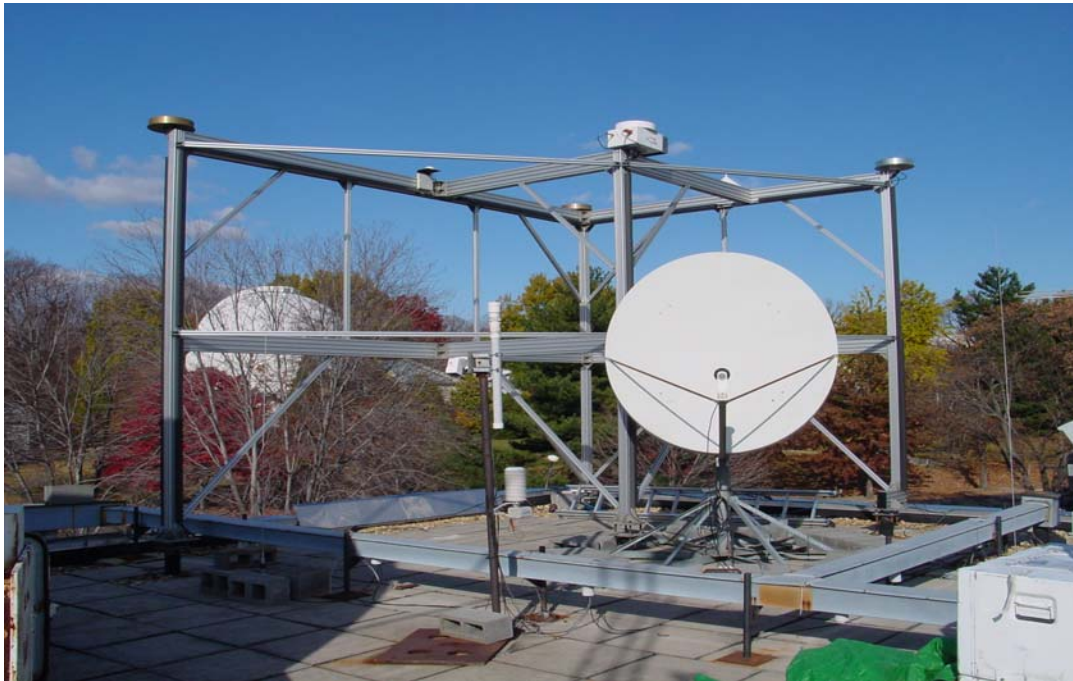
Figure 7. GPS antenna mount, now operational for GPS monitoring, has reduced multipath by roughly a factor of 3. Right of center is a directional antenna used to monitor WAAS signals.
