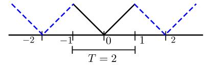
To compute the Fourier series, use (4)-(6) with  $\ell = 1$ . First, observe that f(x) is an even function, so
