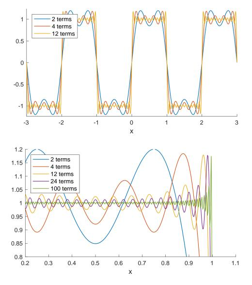
Figure 2: Partial sums for the square wave. Zoomed in figure shows the behavior near the corner at x = 1. Note that the oscillations around the discontinuity do not decrease in size as  $N \to \infty$ .
