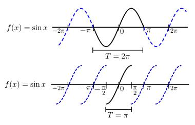
Note that the last two examples show that the periodic extension of a function will depend on the interval chosen and/or period specified. The  $\pi$ -periodic extension of sin x from  $[-\pi/2, \pi/2]$  to  $\mathbb{R}$  is different than the periodic extension from  $[-\pi, \pi]$  to  $\mathbb{R}$ .
