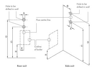
Note: Flue pipe diameter: 150mm 180mm excluding locking bands (see dimension 'A' opposite for hole size).
