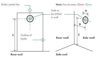
Note: Dimension 'B' is given with the boiler pushed back against the rear wall. Any clearances must be added to 'B'.
