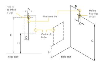
Note: Dimension 'B' is given with the boiler pushed back against the rear wall Any clearances must be added to 'B'.
