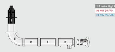
Internal High Level balanced flue kits
