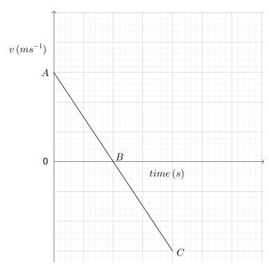
Now we need to describe it. Think about what has happened. Initially the ball is thrown into the air vertically upwards (positive direction) with a speed of  $5\,m/s$ . Point A describes the initial velocity (upward) that the ball has. It is  $5\,m/s$  upward. Then the ball starts to slow down (due to gravity acting on it). This is the part of the graph from A to B. At point B, the ball has zero velocity. It is not moving, and so this is the point of maximum altitude for the ball.
