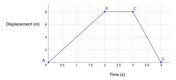
Note that this is displacement (a vector quantity) versus time. Whereas the gradient of the distance versus time graph gave speed, the gradient of the displacement (a vector) versus time graph gives velocity (a vector).
