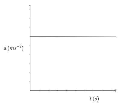
It is simply a horizontal line as the acceleration is constant. The velocity-time graph is shown below.
