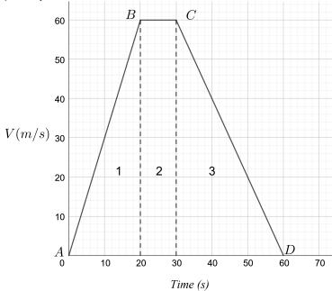
From A to B, the object accelerates from  $0 \, m/s$  to  $60 \, m/s$ . From B to C the object is moving at a constant velocity of  $60 \, m/s$  and from C to D, the object is slowing down from  $60 \, m/s$ . We now look at some features of the graph in detail. In particular we look at the area under the graph and it's gradient.
