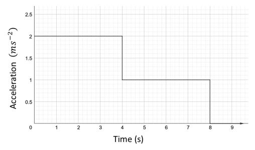
g. Change in velocity is area under the Acceleration-Time graph  $= 8 + 4 = 12 \, m/s$ .
