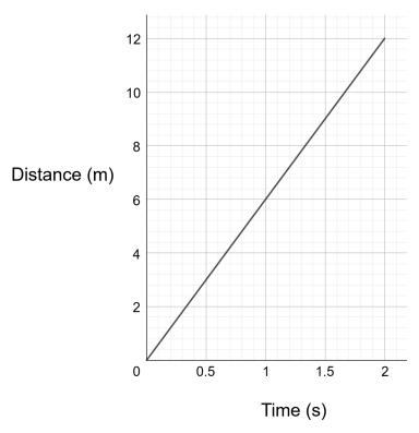
Note that the gradient of a distance (a scalar quantity) versus time graph gives the speed (also a scalar quantity). In this case, the speed is given by
