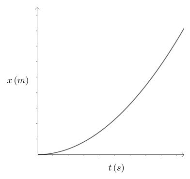
This is a curve. The gradient (slope) at any point on the curve is the velocity at that time. You can find the approximate value of the gradient by drawing a tangent at the point of interest and then calculating the gradient of the tangent.<sup>7</sup>
