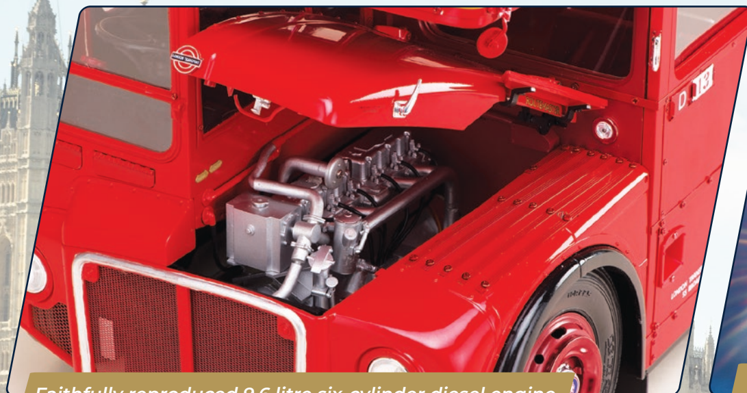
Faithfully reproduced 9.6 litre six-cylinder diesel engine
