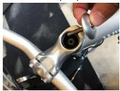
• Slide your stem, with the handlebar attached, off the fork and slide the stem extender in its place.
