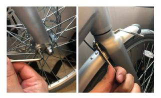
**Step 9:** Install the front light by connecting the cables on the light, to the available white/yellow wire connector inside the frame. If needed, you can cut the zip ties to allow for more cable slack to connect
