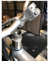
• Use all the included additional rings and slide onto the stem extender.
