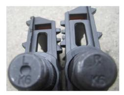
Be careful to not cross thread the pedals. Pro Tip: Pedal threads always tighten towards the front of the bike. (Right pedal has clockwise thread/Left pedal has counter clockwise thread). **PLEASE NOTE: After installing the pedals, make sure to also tighten the crank arm bolts with an 8mm hex wrench. DO NOT RIDE THE BIKE UNTIL THE CRANK ARM BOLTS (circled in red) ARE TIGHTENED DOWN.**
