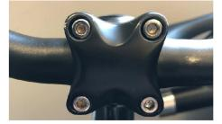
**Step 3:** Align your handlebars using your 5mm hex wrench. Loosen the two stem bolts using your 5mm hex wrench and align the handlebars to be perpendicular to the bike frame. Tighten top bolt first, then the two stem bolts to hold the handlebar position in place.
