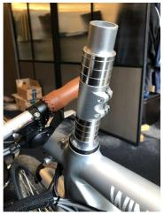
• Slide the stem onto the stem extender, then grab your long bolt and top cap.
