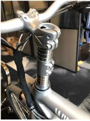
• Tighten down the top cap so that it is firmly securing all the components together.
