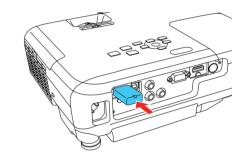
3 Attach the included wireless LAN module cover and secure it using the screw you removed.
