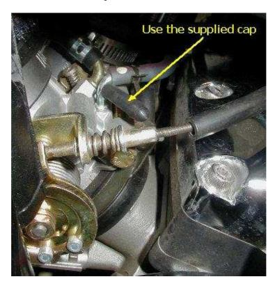
Remove the vacuum hose from rear throttle body nipple. Use the supplied cap and install on nipple.
