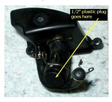
I have indicated where the 1/2" plastic plug should go if you are keeping the stock air box. You can also look in the previous step (picture 4C), where you can disconnect the steel hose and install the plastic plug.
