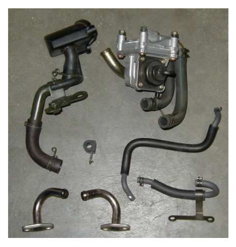
Here is a picture of all my 'Take-Off' parts. If you still have the stock air box, you'll still have the plastic air box extension with the 1/2 plug still attached to the main air box. The steel air hose/bracket would still be discarded.
