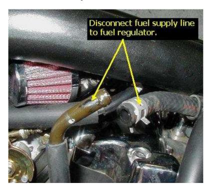
Disconnect the fuel supply line to the Fuel regulator. After this is completed you can set the bracket and fuel regulator aside, to get better access to the elbow fittings on each cylinder.
