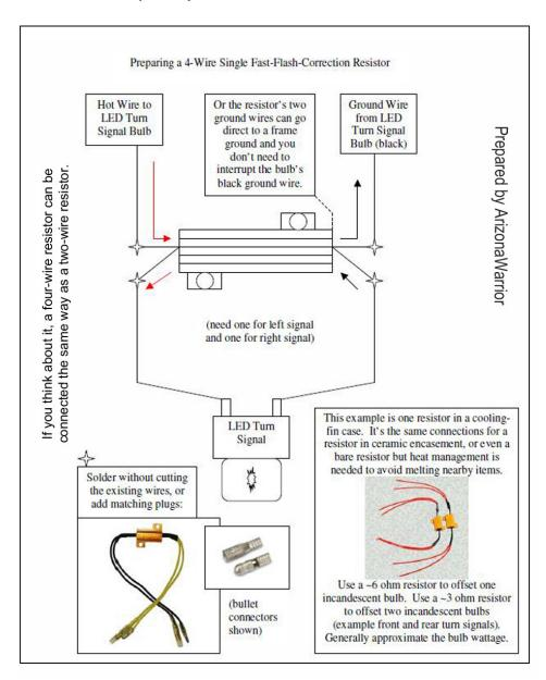
Fast-flash has nothing to do with the front running lights except the filament happens to share the front light bulb.
