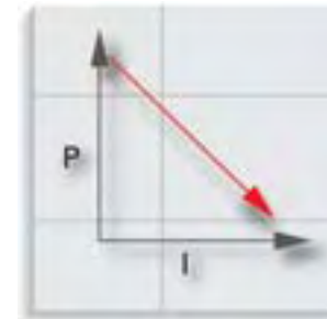
Pressure Control Valves with Falling Characteristic Curve N92, N93, N282 and N283
