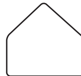
SCHOOL AND SCHOOL CROSSING SIGN
