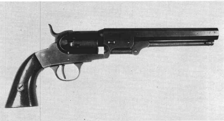
Figure 8 Experimental .31 Caliber 5 shot, 6-inch barrel
