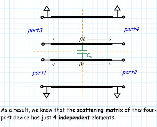
$$\mathcal{S} = \begin{bmatrix} S_{11} & S_{21} & S_{31} & S_{41} \\ S_{21} & S_{11} & S_{41} & S_{31} \\ S_{31} & S_{41} & S_{11} & S_{21} \\ S_{41} & S_{31} & S_{21} & S_{11} \end{bmatrix}$$
