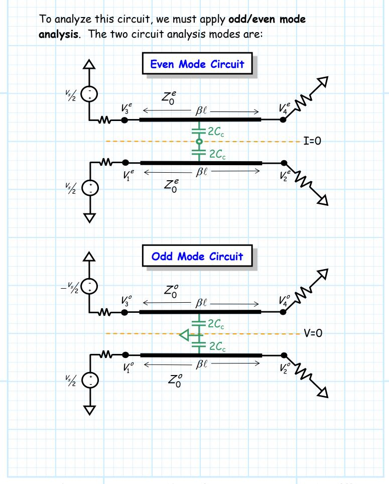
Note that the **capacitive coupling** associated with these modes are different, resulting in a **different** characteristic impedance of the lines for the two cases (i.e.,  $Z_0^e, Z_0^o$ ).
