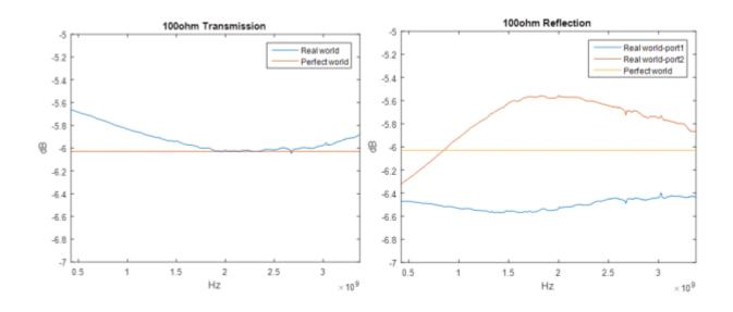
The DUT here is a  $100\Omega$  surface mount resistor, so the ideal result is -6.02dB for transmission and reflection:
