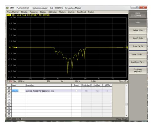
Figure 1: Choosing and naming a blank calibration kit
