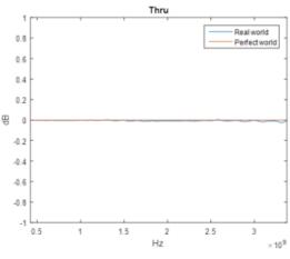
804 from 422 MHz to 3.37 GHz. The Thru standard is used as the normalization reference, so the thru measurement only shows us the repeatability of the calibration kit. Port 1 and port 2's reflection coefficients, S11, when connected to open standard is shown below. Ideally, it should always be 0dB. And the variation here is less that  $\pm 0.1$ dB.
