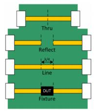
The picture shown above assumes the DUT is perfectly in the middle of the Thru standard. After calibration, the reference plane will be moved from the VNA ports to the two ends of DUT, shown by dashed lines in the picture.
