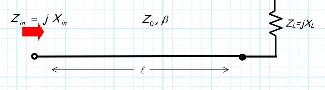
Note that the **opposite** is **not** true: even if the load is **purely resistive** ( $Z_L = R$ ), the input impedance will be **complex** (both resistive and reactive components).
