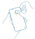
2. Slide the memory card holder until it unlocks, and lift the holder.
