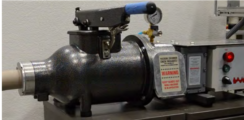
Figure 32. Photo. The pugger mixer used for soil preparation.
