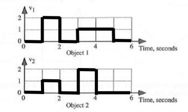
For the 6-second time interval shown, is the displacement of Object 1 in the upper graph (i) greater than, (ii) equal to, or (iii) less than the displacement of Object 2 in the lower graph? \_\_\_\_\_
