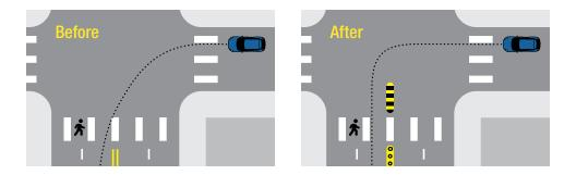
Centerline hardening makes intersections safer for pedestrians by encouraging drivers to make left turns at slower speeds. Bollards and rubber curbs block the diagonal path through the intersection.
