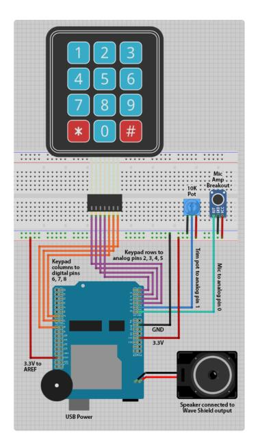
Upload the Adavoice sketch to the Arduino if you haven't already done this. If everything is wired up and loaded correctly, you should head a startup chime when the sketch starts (if using an SD card with the sample WAVs). If there's no sound, use the Arduino serial monitor and watch for diagnostic messages.
