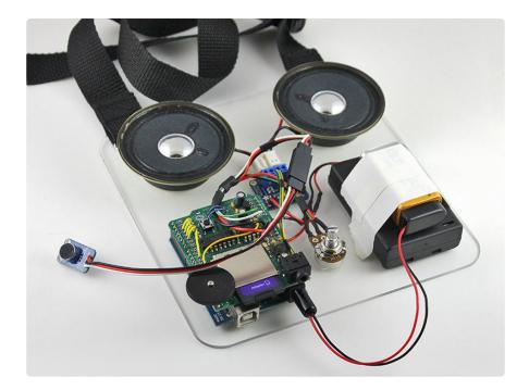
You can run the microphone connection a couple feet to reach inside a mask or helmet. A <u>servo extension cable</u> (http://adafru.it/973) provides a very handy 3conductor separation point, so you can pop your head and set it down! Cut the servo cable in half, soldering one end to the mic amp board and the other side to the Arduino circuit.
