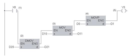
The program is executed from the top to the bottom, when the ladder is branched and ENs and ENOs are connected in parallel.
