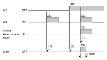
(1) When M0 is off (the conditional formula of the IF conditional statement is FALSE), the on/off determination result will be off. The PLS instruction is not executed. (The M10 remains off.)
