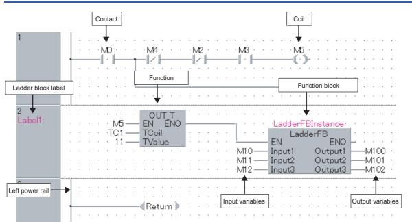
In the structured ladder/FBD language, units of ladder blocks are used for programming. For structured ladder, connect the left power rail and ladder symbols with lines.
