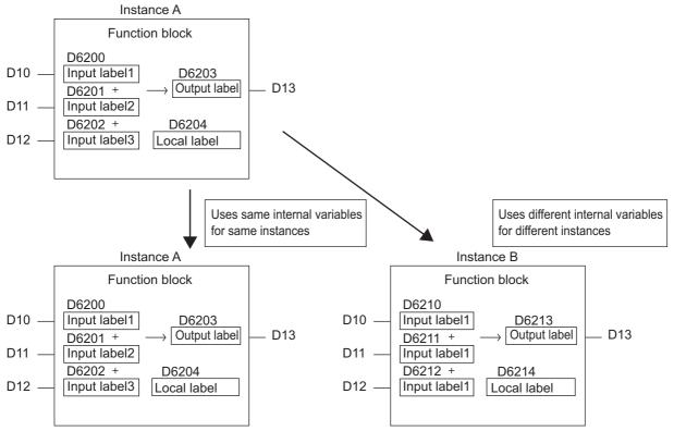
Function blocks perform operations using internal variables assigned to each instance.
