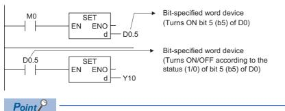
For FXCPU, bit specification of a word device can be used for  $FX_{3U}$  and  $FX_{3UC}$ .
