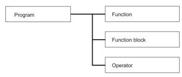
Sequence programs executed in a programmable controller CPU are created by programs of POU. For a simplest sequence program, only one program needs to be created and registered to a task in order to be executed in a programmable controller CPU.
