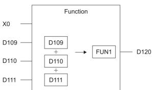
A function block uses internal variables. Different devices are assigned to the internal variables for each instance of function blocks.
