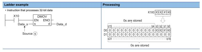
When digits are specified at the destination (d), the points by the specified digit are the target of destination. (Data\_d1:K5M0, Data\_d2:K5M10, Data\_s:D0) Bit devices below the number of points designated as digits do not change.
