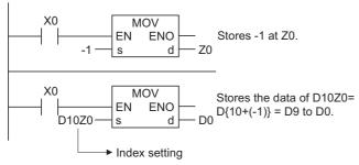
\*1 For the specifications of the index register, refer to the User's Manual (Function Explanation, Program Fundamentals) for the CPU module used.
