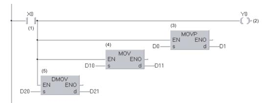
The program is executed in the order as shown below when the MOV instruction (4) in the above figure is moved to the top.
