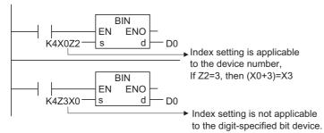
For intelligent function module devices<sup>\*1</sup>, an index setting is applicable to both start I/O numbers of the intelligent function module and buffer memory addresses.
