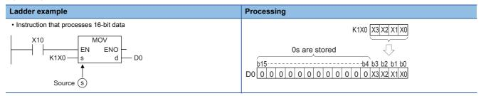
When digits are specified at the destination (d), the points by the specified digit are the target of destination. The status of bit devices which follow the digit-specified bit devices is not changed.
