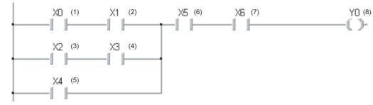
The program is executed from the left power rail to the right when the ladder is not branched and ENs and ENOs are connected in series.
