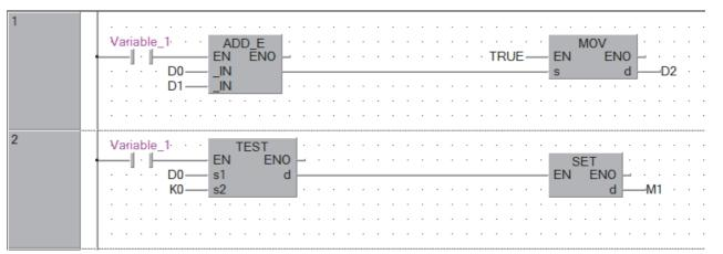
When Variable\_1 is OFF, the MOV or SET instruction is executed though the ADD\_E or TEST instruction is not executed. Even though Variable\_1 is OFF, a value may be set in D2 by the MOV instruction or M1 may turn ON by the SET instruction.
