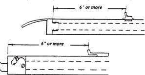
Fixed rear open sights may have no mechanical means of adjusting the elevation or windage, and therefore are non-adjustable in nature. Adjustable rear open sights may have a mechanical means of adjusting elevation and windage.
