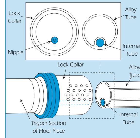
the floor piece. Insert the alloy tube into either end pieces ensuring the small diameter internal tube lines up with the nipple inside the end section (see illustration).
