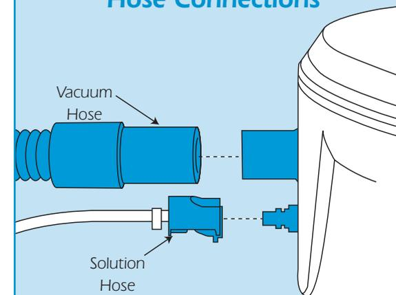
solution supply hose to both machine and cleaning wand (or to the upholstery cleaning head).
