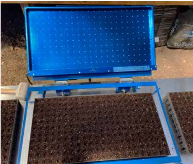
FIGURE 16. Vacuum seeder in operation with pelleted lettuce seed held in place and ready to drop into the tray.
