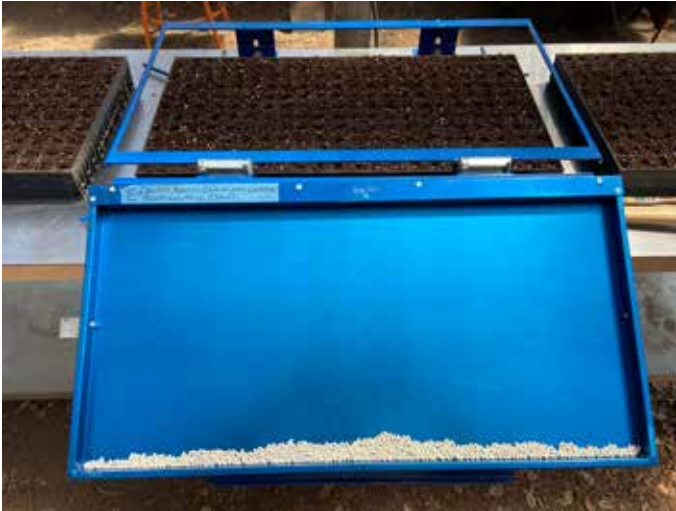
FIGURE 15. Vacuum seeder seed plate with loose pelleted lettuce seed before distribution to each seed hole.
