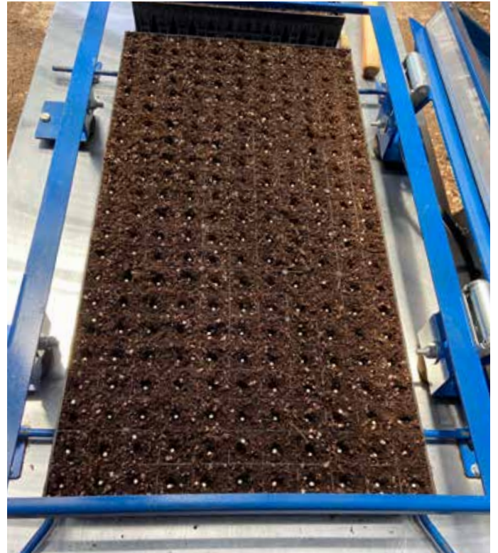
FIGURE 17. Pelleted lettuce seed just sown using vacuum seeder into pre-dibbled 242 tray.
