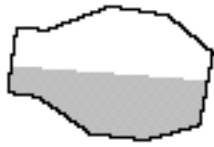
Less than capacity load in drum
